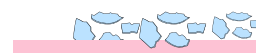
The cold solution is poured to obtain the crystals by pressing them between the sheets of filter paper
